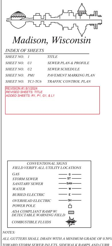
ALL GUTTERS SHALL DRAIN WITH A MINIMUM GRADE OF 0.50% TOWARD STORM SEWER INLETS. SIDEWALK RAMPS AND CURB THRU SIDEWALK RAMPS SHALL HAVE A MAXIMUM SLOPE OF 1" PER 12", SIDEWALK AND CURB RAMPS SHALL BE CONSTRUCTED WITH A SIDE SLOPE OF 1.50%. SIDEWALK SHALL HAVE A MINIMUM LONGITUDINAL SLOPE OF 0.50% AND A MAXIMUM LONGITUDINAL SLOPE OF 5.00% EXCEPT WHERE STREET GRADES EXCEED 5.00%.
